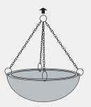
> Mirrors are to be hung from the ceiling and are supplied 4 chains each of 1 metre in length which are joined at a central point
